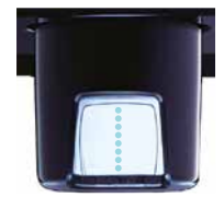
8 sensors measure while moving left to right
