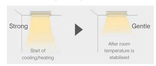
In addition to the conventional 4 fan speed settings, units are now equipped with an Automatic Air-Speed Adjustment Mode. This setting automatically adjusts the air-speed to conditions that match the room environment. At the start of heating/cooling operation, the airflow is set to high-speed to quickly heat/cool the room. When the room temperature reaches the desired setting, the airflow speed is decreased automatically for comfortable heating/cooling operation.
